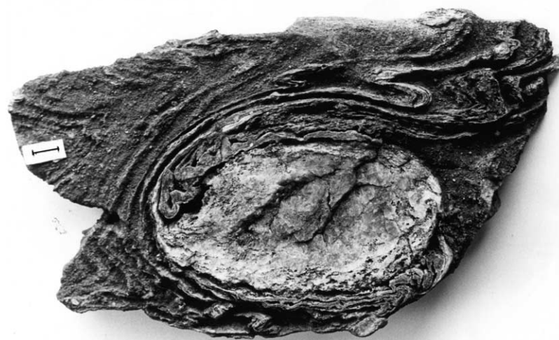
Fig. 13. Horizontal oval section of an elongate pegmatite clast. This section is parallel to E_2 and E_3 of our nomenclature of Fig. 15. The mylonitic foliation in the neighbourhood is asymmetrically deformed with embaying folds forming isoclinal overturned structures suggesting a rotation of 180^\circ . In foliation-parallel sections the long-axis (i.e. E_1 axis) of the cylindrical clast is elongated to at least few tens of decimetres along the down-dip direction of stretching lineation. Scale bar 1 cm.
